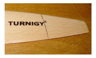
"The reason we measure pitch at 75% of the diameter is two-fold. Generally, the pitch of a propeller is not completely constant, varying somewhat from hub to tip to optimize it for the different linear speeds at each point along the blade. The pitch at 75% corresponds roughly to the average effective pitch of the propeller. Secondly, the propeller is sufficiently wide at 75% to allow one to get reasonably accurate measurements of blade width and height."
